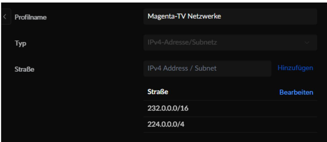
The screenshot shows the UniFi controller interface for configuring a network profile. The profile name is 'Magenta-TV Netzwerke'. The type is set to 'IPv4-Adresse/Subnetz'. The 'Straße' (Address) field contains two entries: '232.0.0.0/16' and '224.0.0.0/4'. There are buttons for 'Hinzufügen' (Add) and 'Bearbeiten' (Edit) next to the address field.
